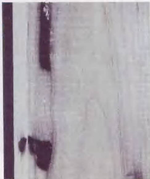
Worm holes: Most insects attack the tree or log just below the bark layer.
